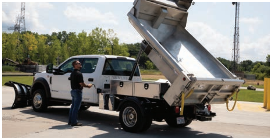
The best equipment purchases are those that do double duty. This truck is outfitted as a dump truck for spring, summer and fall, and a salt spreader for the winter.
